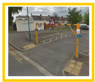
Single Leaf Opening Height Restriction Barrier can be opened to allow access for all vehicle types when necessary. When locked in the closed position, this is a highly effective deterrent to prevent high sided vehicles entering or gaining access to the carpark. This is a very popular option with local authorities, shopping centres, train stations and public carparks.
