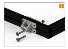
Where there will be a drop bolt mounted, it is necessary to insert the head of the bolt on the inside of the leaf. In all other places, fit the bolts such that the head of the bolt is on the exposed face of the gate. This results in the nut being protected from any tampering as it is shielded by the mesh/hoarding panels.
